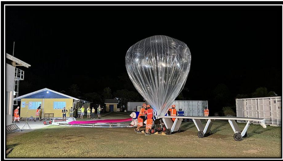
Researchers prepare to launch a Strateole-2 balloon with sensors capable of detecting earthquakes from thousands of kilometers away.
