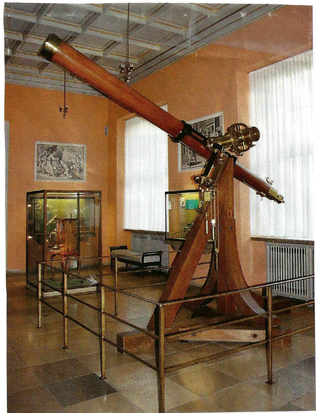
DISCOVERY TELESCOPE Johann Galle discovered Neptune using this beautiful 9-inch Fraunhofer refractor, which is currently on display at the Deutsches Museum in Munich.
